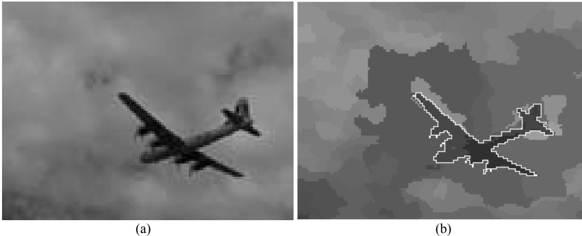
Figure 3. (a) The original image, (b) Segments obtained by mean shift (different grayscale levels) and the clustering boundary after merging according to the Boltzmann distribution (bright white curve).
