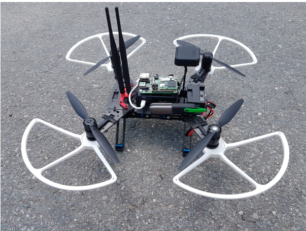
Figure 10: HIRO-NET aerial node prototype.
