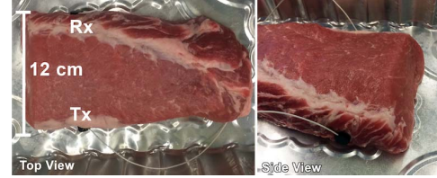
Fig. 21. Experiment setup for porcine meat scenario along 12 cm.
