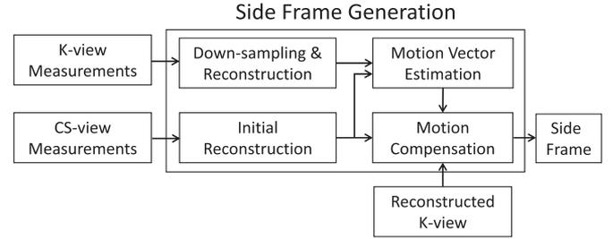
Fig. 2. Block diagram of side frame generation.
