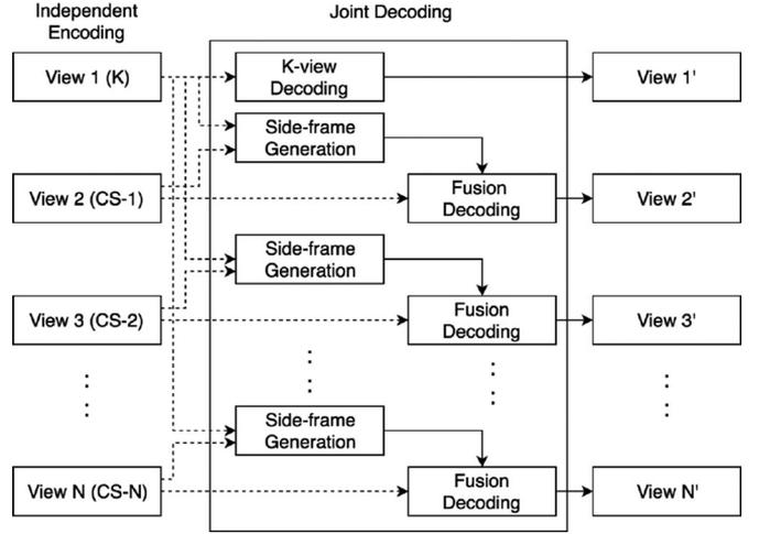
Fig. 1. Multiview encoding/decoding architecture.
