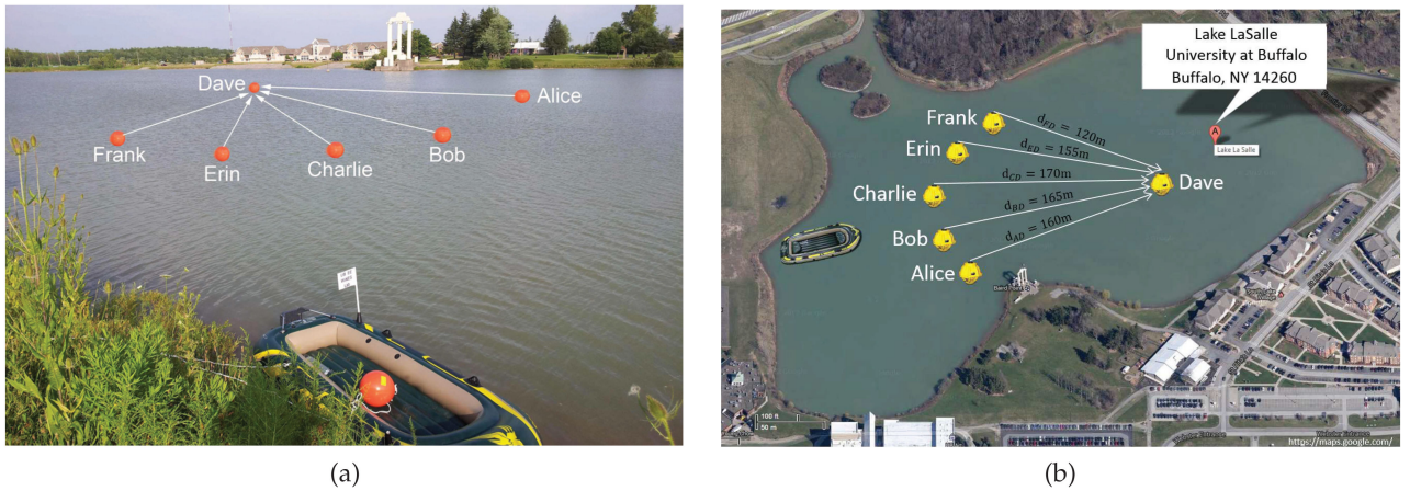
Fig. 6. (a) Deployment of the six underwater acoustic modems in Lake LaSalle at the University at Buffalo; (b) Aerial view of the underwater acoustic testbed.
