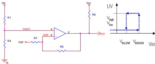
Figure 6 Under-Voltage Sense Circuit with Hysteresis
