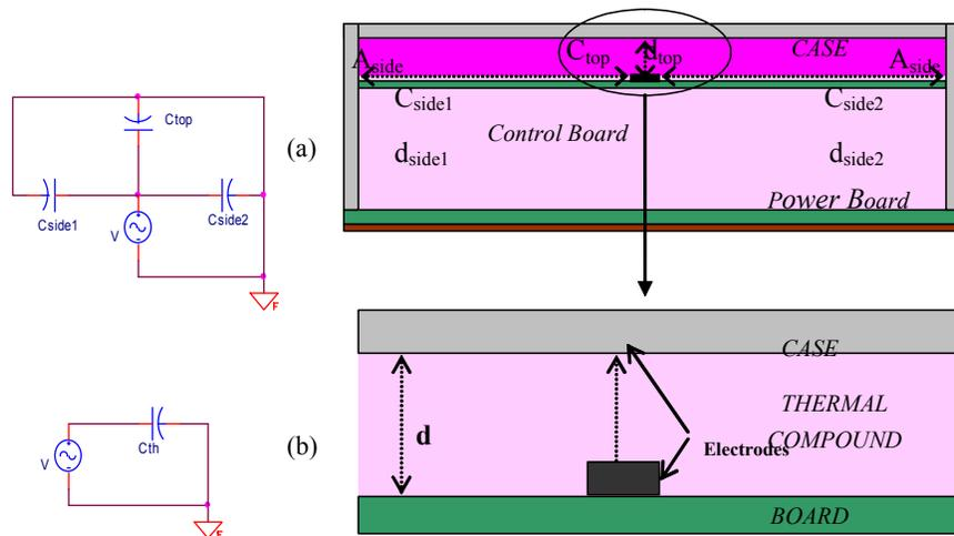
Figure 10. Proposed method to be studied to analyze capacitive effect,  $C_{th}$  on the resistor when adding an enclosure
