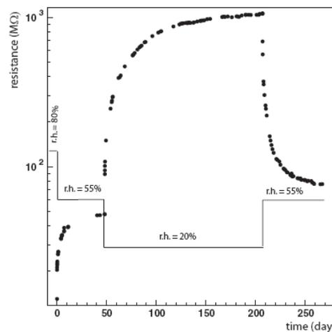
Figure 2. Bakelite resistance change at 25C and different relative humidity [8].
