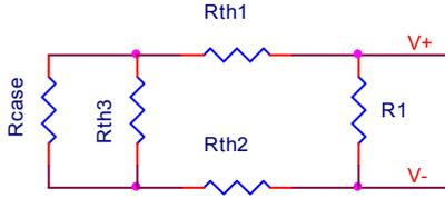
Figure 5. Equivalent resistive model of paths in Fig. 4
