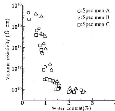
Figure 1. Dependence of Volume resistivity ( $\rho_v$ ) of epoxy composites on water content.[7]
