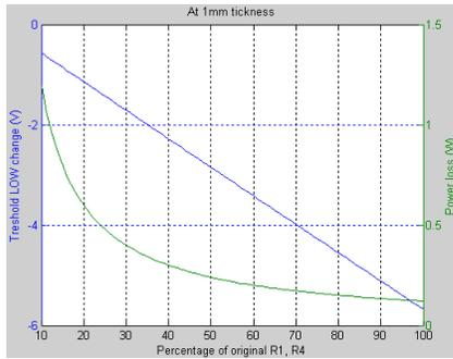
Figure 9. Under-voltage threshold and Power Loss for different values of R1 and R4 at 1mm thermal compound thickness with 0.8% water content.
