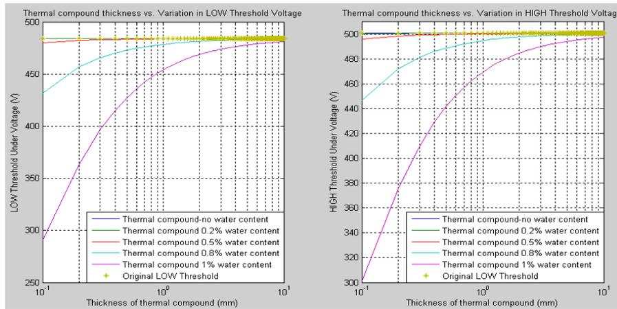
Figure 8. Variation in  $V_{thLOW}$  and  $V_{thHIGH}$  in under-voltage lockout circuit, using thermal compound at 25°C
