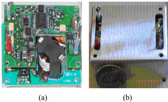
Figure 3. Half-bridge converter with (a) and without (b) compound and aluminum enclosure
