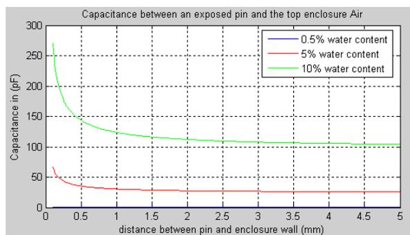
Figure 12. Capacitance between exposed pin and enclosure-free air
