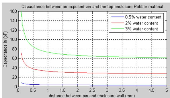
Figure 11. Capacitance between exposed pin and enclosure-rubber
