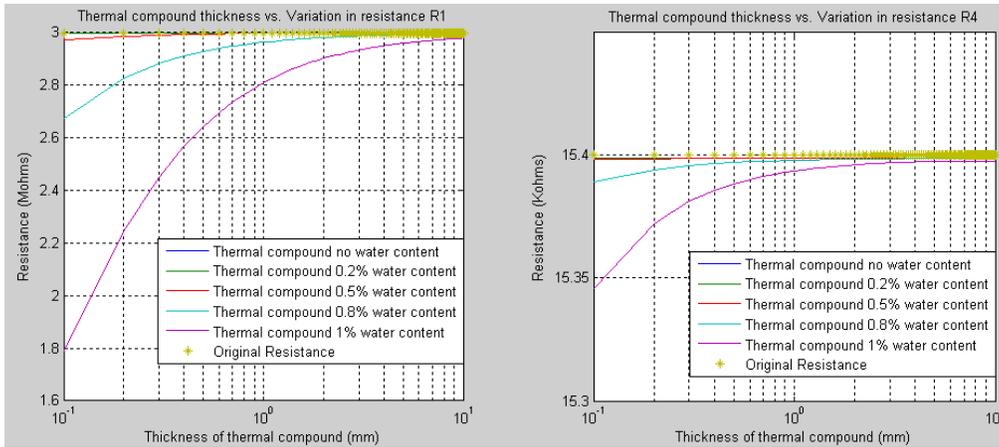
Figure 7. Variation in resistance R1 (a) and R4 (b) using thermal compound at 25°C
