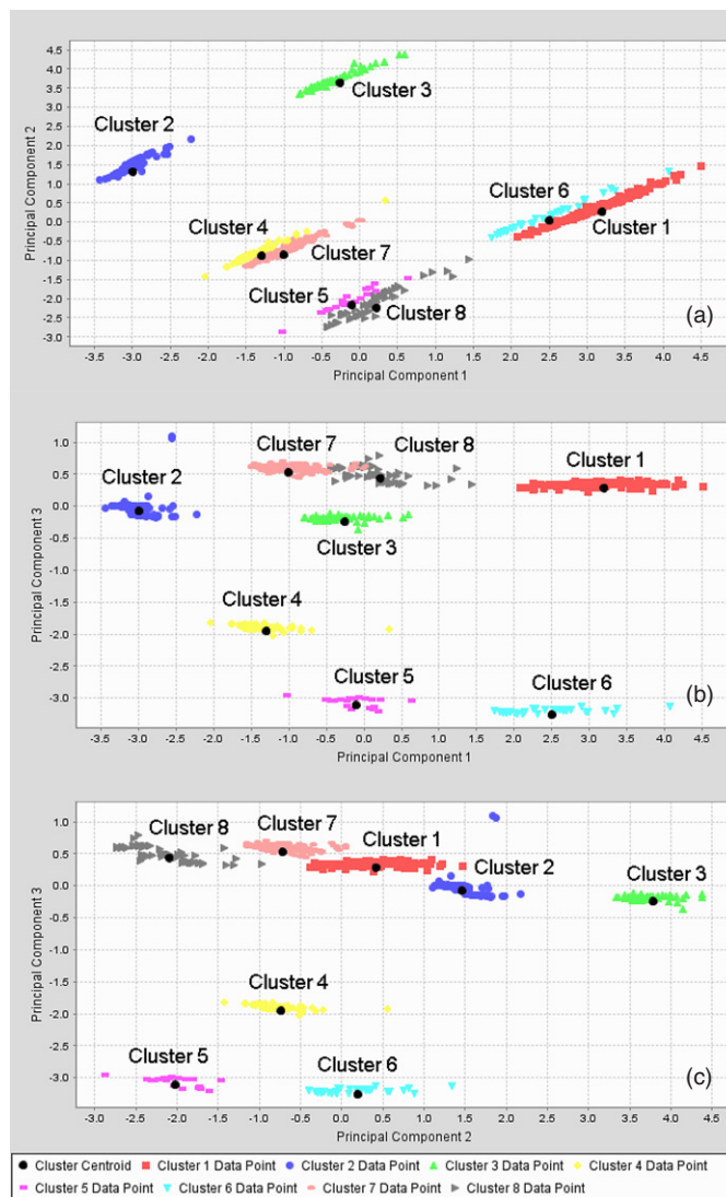
Figure 2. The training data projected onto two-dimensional planes formed by two of its first three principal components: (a) principal components 1 and 2; (b) principal components 1 and 3; (c) principal components 2 and 3.
