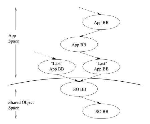
Figure 3: BB Execution path: from the application to a shared object
