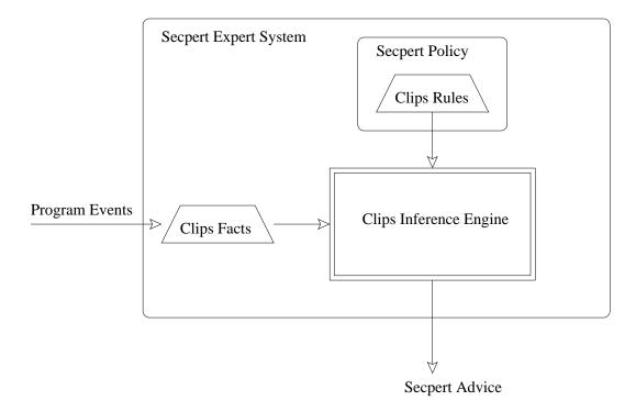
Figure 2: Secpert Expert System architecture
