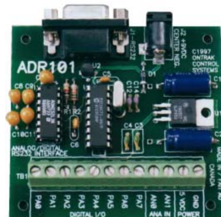
Fig. 3. Ontrak ADR101 serial data acquisition interface (using RS232).
