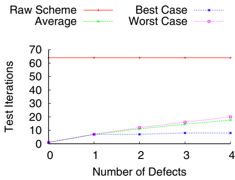
Fig. 4: Comparison of best, average, and worst number of test iterations in proposed scheme to Raw Testing Scheme
