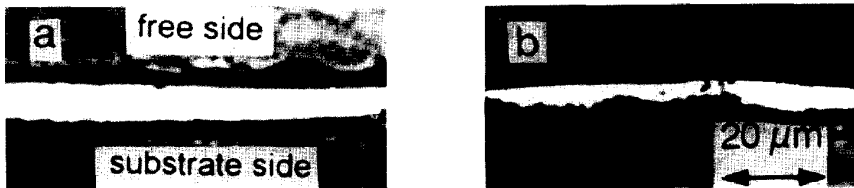
Figure 10. Metallographs of the \text{Fe}_{33}\text{Zr}_{67} alloy ribbons: (a) as-quenched; (b) partially crystallized.
