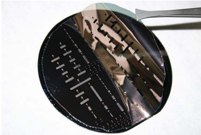
Figure 8: Wafer scale patterning using a flexible parylene shadow mask.
