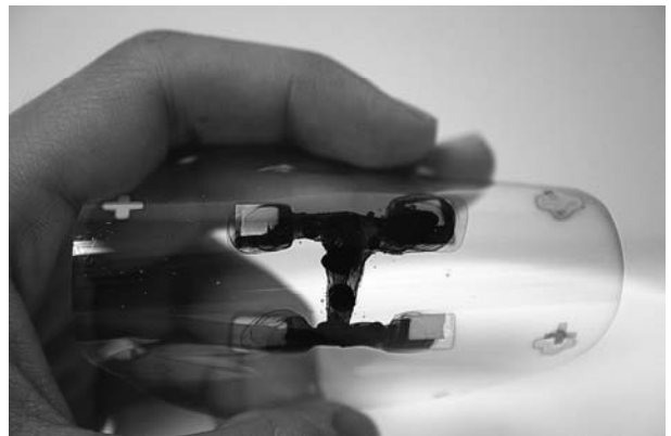
Fig. 1 Optical photograph of the CNT-parylene sandwich-films
