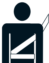
The wrong way to wear a safety belt.
