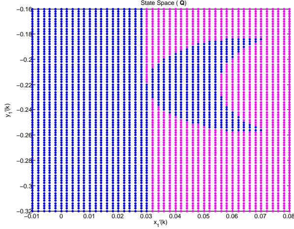
Fig. 3. Partitioning of the state space. Red is \theta_1 (PROCON; not visible in this figure), purple is \theta_2 (LINCON), blue is \theta_{34} (OTHER).
