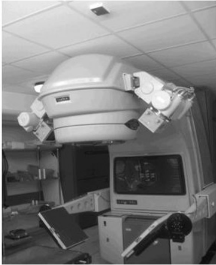
Figure 3: The Integrated Radiotherapy Imaging System (IRIS), used as the hardware platform for the proposed gating technology in this paper.
