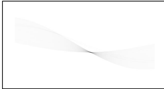
Figure 35 - HT(\theta, \rho) of B(x,y) from figure 35. Maximum response at \theta = 7 degrees
