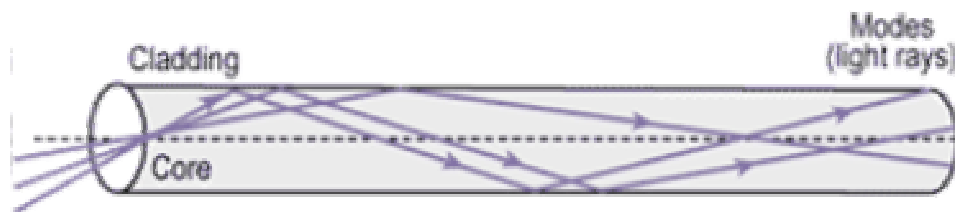
Figure 9: Light Mode Propagation in Multimodal Fiber
