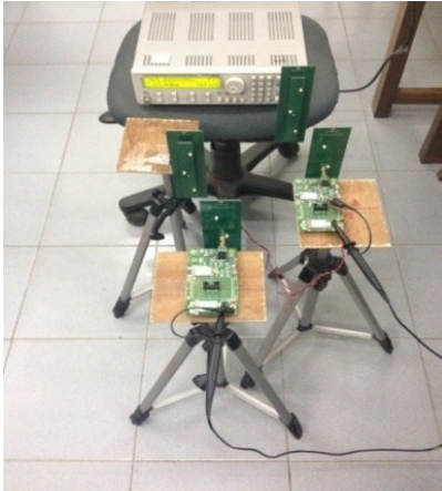
Figure 2. Experimental set-up for finding the optimal position for the intermediate node.
