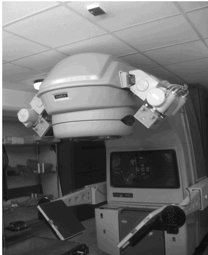
Figure 1. The integrated radiotherapy imaging system (IRIS), used as the hardware platform for the proposed gating technology.
