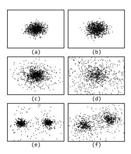
Figure 10. I/Q constellation in Setup A for devices D1 and D2; (a) D1 before FFT, (b) D2 before FFT, (c) D1 after FFT, (d) D2 after FFT, (e) D1 Equalized, (f) D2 Equalized.
