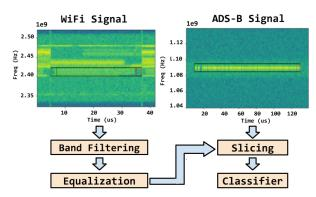
Figure 5. Pre-processing and Classification Pipeline. For WiFi transmissions (left), we perform band filtering (i.e., extracting the signal shown by the bounding box). The sliding window creates multiple slices that are fed to the classifier for training and testing.
