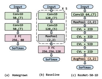
Figure 1. The CNN architectures used in this Paper.
