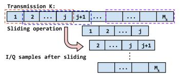
Figure 2. Given a time-series of length  $M_k$ , we create  $M_k - j + 1$  subsequences of length j by sliding a window of length j over the larger sequence (or stream) of I/Q samples (with stride 1). This leads to inputs of a fixed length, but also enhances shift invariance.
