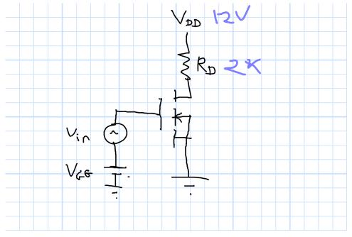
For two cases, draw the load lines on the figure and write the equations for calculating the DC drain current,  $I_D$ . Remember that you can neglect the Early effect at this point.
