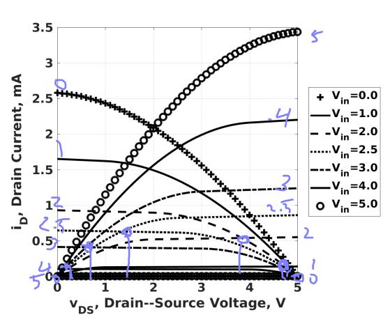
From the given transistor curves for a CMOS logic inverter in the figure above, draw the transfer function. Be sure to show numbers on the axes.
