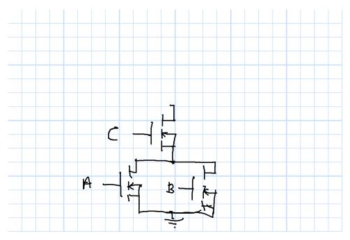
The figure shows the pull–down portion of a logic gate with three inputs. For all possible combinations of true and false inputs, show show whether the pull–down circuit is open or shorted.
