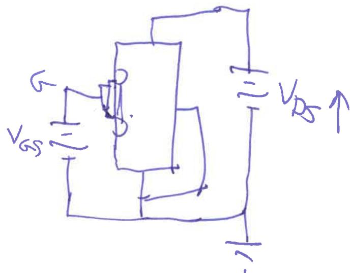
$$i_D = K (V_{GS} - V_{TO})^2 \\ \text{Saturation}$$
