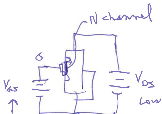
$$i_D \propto (V_{GS} - V_{TO})$$
