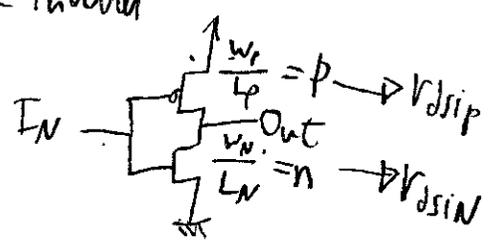
The series resistance of the transistors in the gate should sum up to an equivalent resistance  $\leq r_{dsip}$  (or  $\leq r_{dsin}$ ) for all input combinations, where the series resistances of the transistors between the output  $V_{out}$  and  $V_{DD}$  (or ground) are added when the transistors are "turned on".
