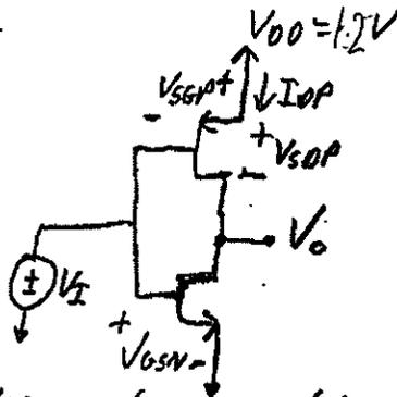
It is required that  $V_o = \frac{V_{DD}}{2} = 0.6 \text{ V}$ , which implies that  $I_{OP} = I_{ON}$
