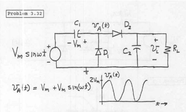
Notice that  $C_1$  and  $D_1$  form a clamp circuit. Furthermore,  $D_2$  and  $C_2$  form a peak rectifier so the load voltage is approximately equal to  $2V_{\rm m}$  which is why this circuit is called a voltage doublem.
