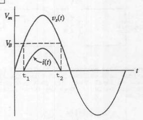
Peak current flows at the instant for which  $\boldsymbol{v}_{\text{S}}(\text{t})$  attains its maximum value. The maximum current is
