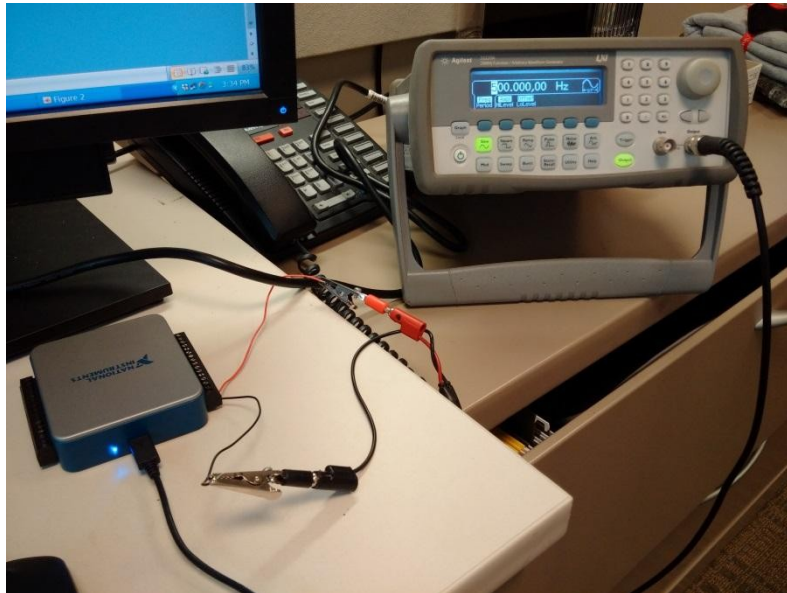
Figure 3. Connecting the Function Generator to the DAQ Board
