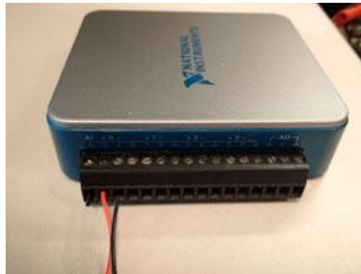
Figure 2. Connecting Wires to the DAQ.
