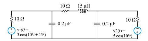
Por this circuit, apply the **Node-voltage method** in phasor domain to give two systems of equations and two unknowns node voltages **VN1** and **VN2** (indicate these on the figure above). Write these, simplify and put in matrix form below. Place a box around your final answer to make it easy for a grader to find. YOU DO NOT HAVE TO SOLVE VN1 and VN2. (8 Points)
