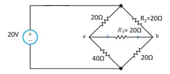
(a) Write node-voltage equations for this circuit. Simplify these equations and then put the system of equations in matrix form. You do not need to solve for the values of the node voltages.
