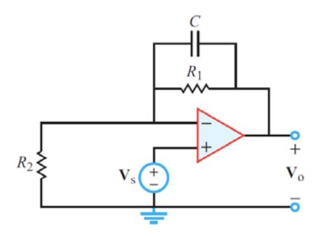
(a) In the circuit above, if  $V_s$  and  $V_o$  are phasor voltages, find the ratio  $V_o/V_s$  as a function of frequency by using the ideal op-amp model and expressions for the impedances of the circuit element. Put a box around your final answer so it can easily be found by a grader.
