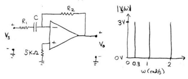
Extra Credit: (5 pts) Derive the frequency at which the transfer function  $H(\omega) = \frac{V_0}{V_i}$  of the following circuit is equal to zero.
