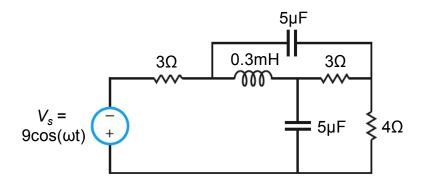
3B) Application of the **mesh-current** method in phasor domain will yield a system of three equations for three unknown phasor currents. **Write** and s**implify** these equations and then put the system of equations in **matrix** form. **You do not need to solve for the values of the three currents.** (14pts)
