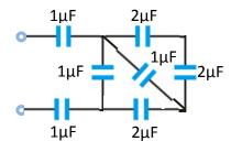
1D) What is the equivalent Impedance ( $Z_{eq}$ ) of the following network if the source has an angular frequency of 1000 rad/s (4pts)
