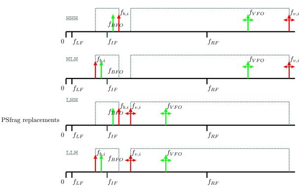
(1.b) (20/100 pts.) Any design with  $X_3 = H$  yields an IF image rejection filter with a wider bandwidth. Any one of the following four graphs is an acceptable answer.
