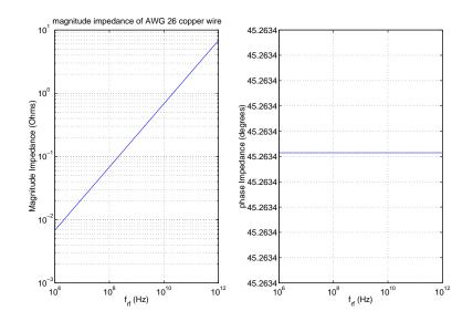
Figure 1: Impedance plots of AWG 26 copper wire.
