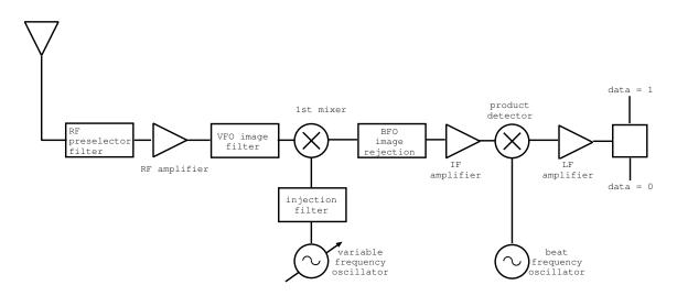
Figure 1: Superheterodyne receiver structure.
