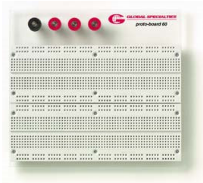
Front-side view of a proto-board showing the tie points arranged in rows and columns
