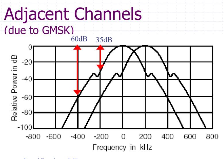
Specification: 9dB In practice, due to power control and shadowing, adjacent channels Cannot be used within the same cell...
