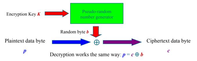
*Thought experiment 1*: what happens when  $p_1$  and  $p_2$  are encrypted under the same "random" byte **b**?
