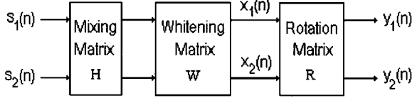
Fig. 1. System block diagram for two sources/observations.
