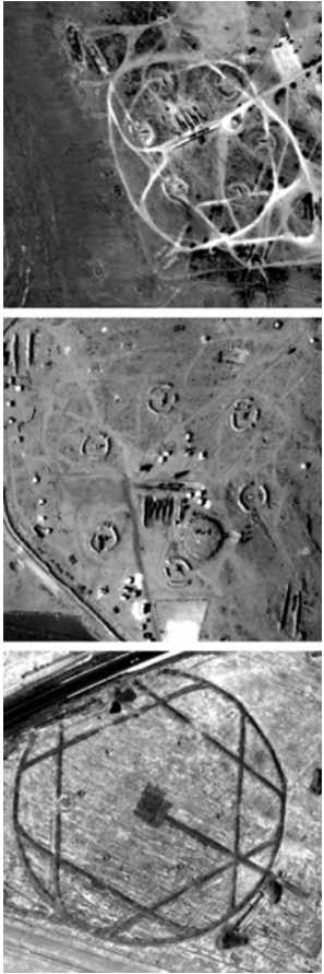
Figure 6: Examples of surface to air missile sites (SAM) -- targets sought by participants. SAM sites typically consist of a few missile launchers in a radial arrangement, with paths linking them.
